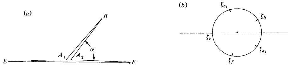
FIGURE 2. The conformal transformation. (a) The z -plane. The physical boundary may be thought of as a degenerate polygon. (b) The \zeta -plane. The boundary in the z plane may be transformed into the unit circle in the \zeta -plane via equation (2.1).
